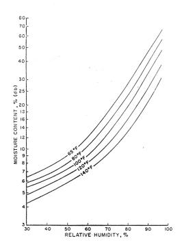
Fig. 3. Equilibrium moisture content as a function of temperature and relative humidity from combined data of Jeffrey (1940) and Locklair, <u>et. al.</u> (1957).
